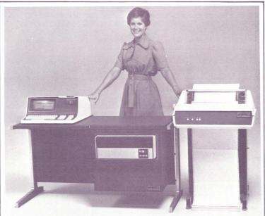
The Datapoint 4520 includes a 48K processor, 2.5/2.5 MB disk storage, multiport adapter, and system software. Optional belt printer shown.
